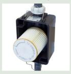
3 Replace the RFC 911 filter element
